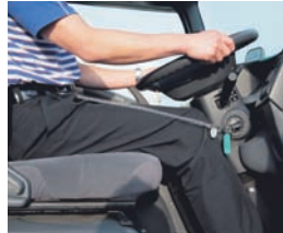
The initiative for eliminating idling by removing keys began in 1997. If the driver does not remove the key, he is unable to leave the driver's seat.
