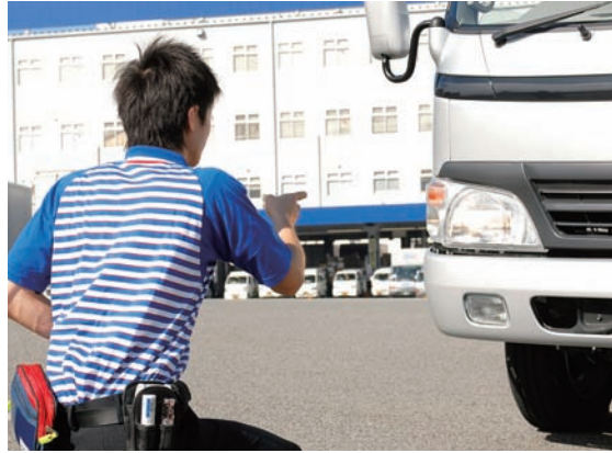
The routine inspections are performed every morning. More rigorous inspections are held once every three months and once a year, along with regular maintenance.
