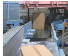
The automatic sorting line winds around a large installation. Packages are dropped into a series of chutes situated around the conveyor.
