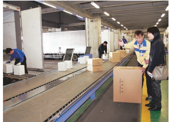
The automatic sorting machine appears in the foreground, while the manual sorting line can be seen in the back. Employees work skillfully and with little wasted motion.
